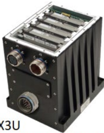
Air Cooled Packaging [VITA 48.1] Standardized Universal 6U VPX PCBA
